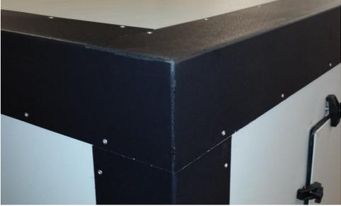
The **base frame** constitutes a continuous support to the units under all sides and allowing to unload the weight on a larger surface reducing the load on the structure on which our units are placed. The base frame is manufactured by coupling a galvanised cold-rolled metal profile, 30/10 thickness welded at the corners and with a height of 180mm.
