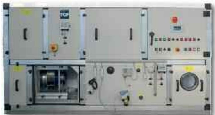
The whole control and power system is installed and wired on board the unit in the factory, to be then tested and thoroughly checked before despatching. The power and control board are made from a metal box with protection class IP65. The LCD display is illuminated from behind and the signal LED lights allow a quick and immediate view of the state of the AHU.
